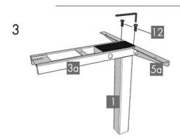
The Frame End-CB (part 3a) should be placed on the side of the desk where you plan to mount the Control Box (part 6) and the Handset (part 7).
