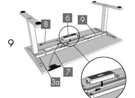
Connect the cable exiting the Leg (part 1) that is attached to the Frame End-CB (part 3a) directly into the Control Box (part 6). Attach the Control Box(part 6) to the underside of the desktop using four(4) M5x20 Wood Screws(part 13).
