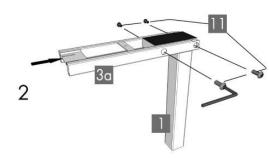
Place one of the Legs (part 1) into the Frame End-CB (part 3a) ensuring that the bar (arrow) is on "top" in relation to the Leg (part 1).
